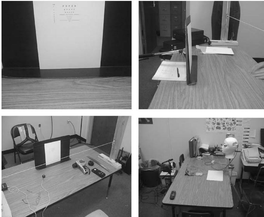
Figure 1 Various photos of the test room showing the desk, eye chart in place and in enlargement, the manikin head and video camera. Note that for both the pupil size measurements and related calibration the camera was moved from the position shown and placed on the table with the lens at the eye chart position
